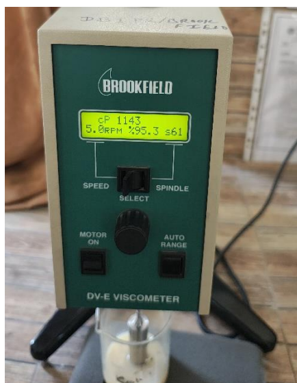
Figure 7: Viscosity of emulsion using Brookfield viscometer.
